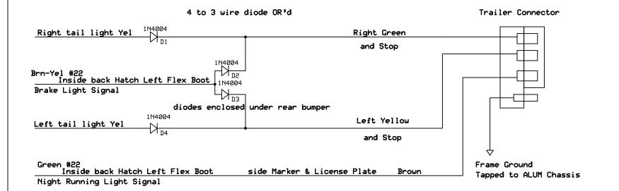
Two #22 wires soldered/heat shrink to sheathed dual conductor routed through left vehicle frame channel
