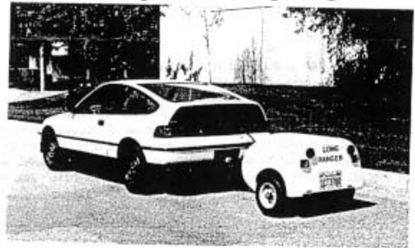
The Long Ranger is a compact, lightweight trailer housing a small internal combustion engine and generator. The aerodynamic trailer is towed behind the electric vehicle enabling the driver to extend his range by 200 miles per 5 gallon tank of fuel. It is also completely detachable, making it possible for the car to remain primarily a zero emissions vehicle. With the addition of the Long Ranger, electric vehicles are not limited to "local commuter" status anymore.
