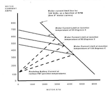
Fet junction temperature refers to the internal transistor junction. During operation, the junction temperature is always greater than the heat sink temperature. Cooling the heat sink will help reduce temperature of the junctions.
