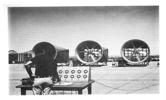
Fig. 6 Three of Eight Units of the NHTSA Crosswind Generator
