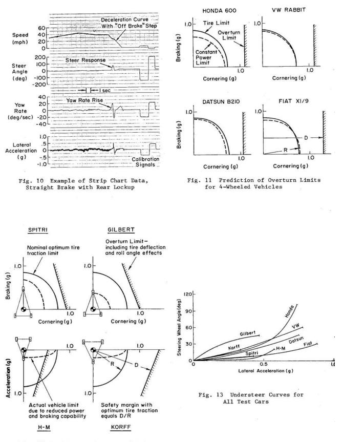
Fig. 12 Prediction of Overturn Limits for 3-Wheeled Vehicles
