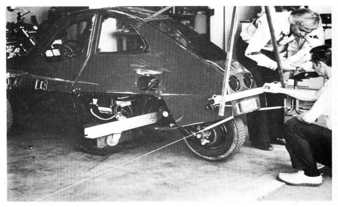
Fig. 7 Measurement of the Vehicle Polar Moment Using the Torsional Pendulum Frequency Method
