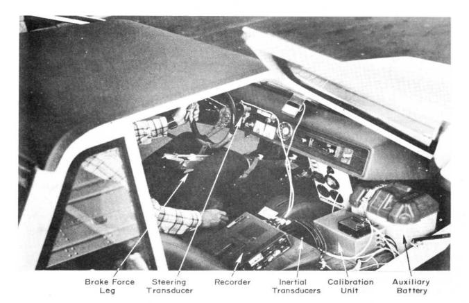
Fig. 9 Placement of Instrumentation in Test Vehicle
