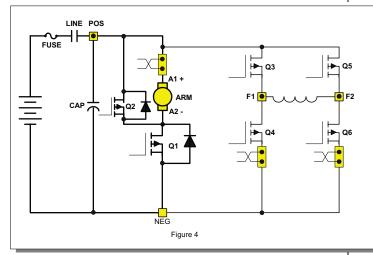
By energizing the transistors in pairs, current can be made to flow in either direction in the field. The field and armature control circuits typically operate at 12KHZ to 15KHZ, a frequency range normally above human hearing. This high frequency, coupled with the elimination of directional contactors, provides for very quiet vehicle operation.
