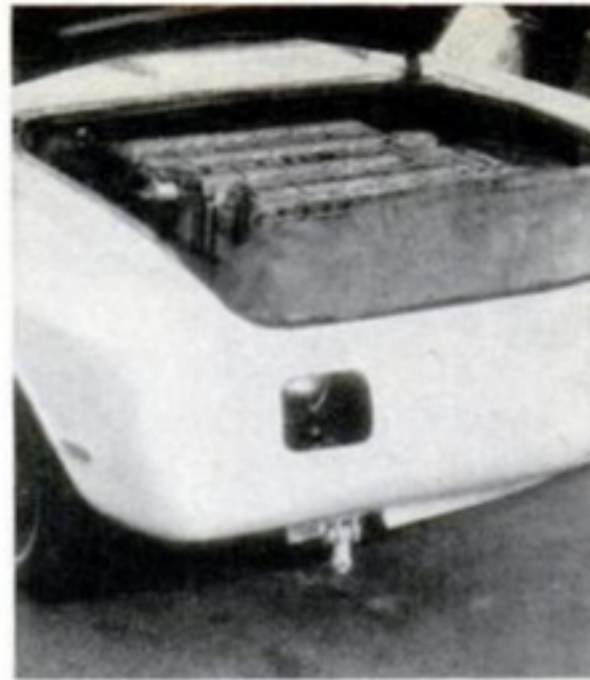
BACK SEAT AND FRONT BOOT contain 320 cells arranged in four, 80-cell, 100-volt packs. Headlight cutouts are also cooling-air scoops
