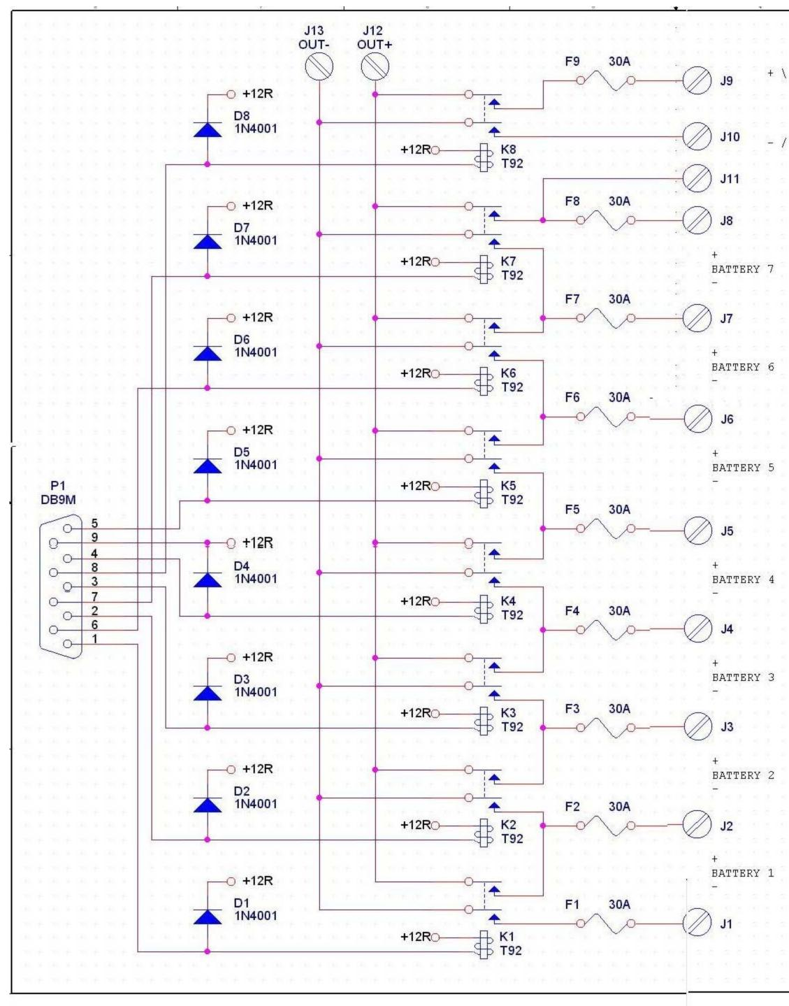
This is the schematic for the relay board of Lee Hart's battery balancer. Again the file is big, to show the details.
