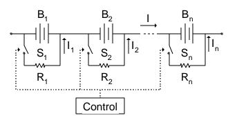
Figure 9. Dissipative Method
