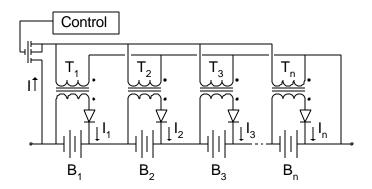
Figure 8. Multiple Transformer
