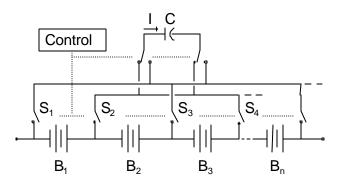
Figure 2. Flying Capacitor Charge Shuttling Method
