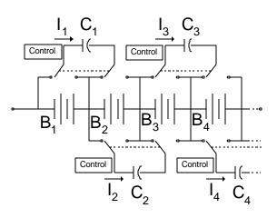
Figure 4. Charge Shuttling with Several Cells
