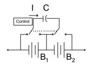
Figure 3. Charge Shuttling Between Two Cells
