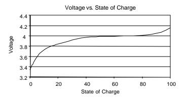
Figure 5. Open Cell Voltage of Lithium Polymer Battery
