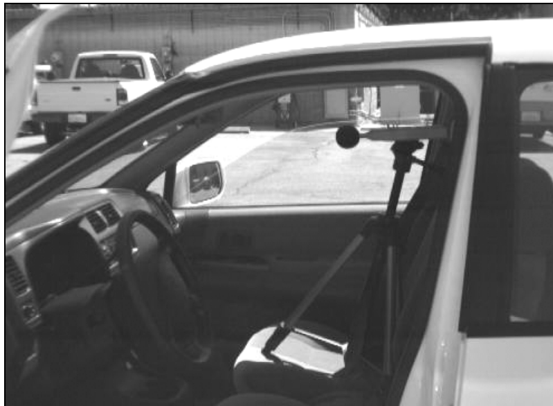
Figure 5-11. Sound level meter positioned to measure sound intensity at ear level.
