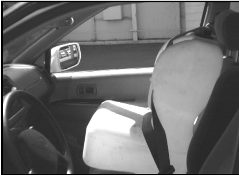
Figure 6-1. Water dummies used in load tests.
