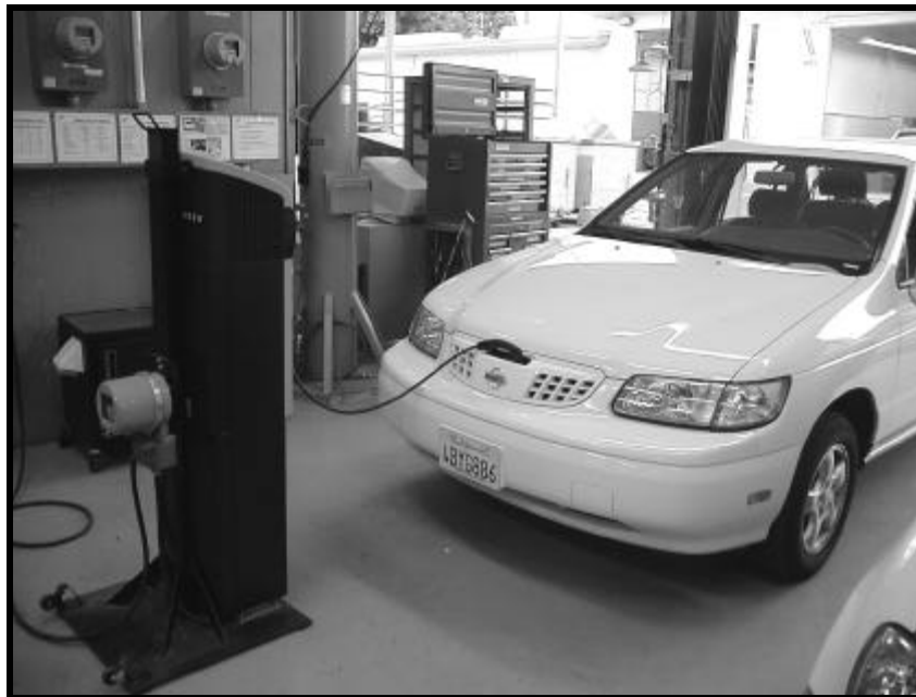
Figure 5-1. The Altra-EV uses inductive charging.
