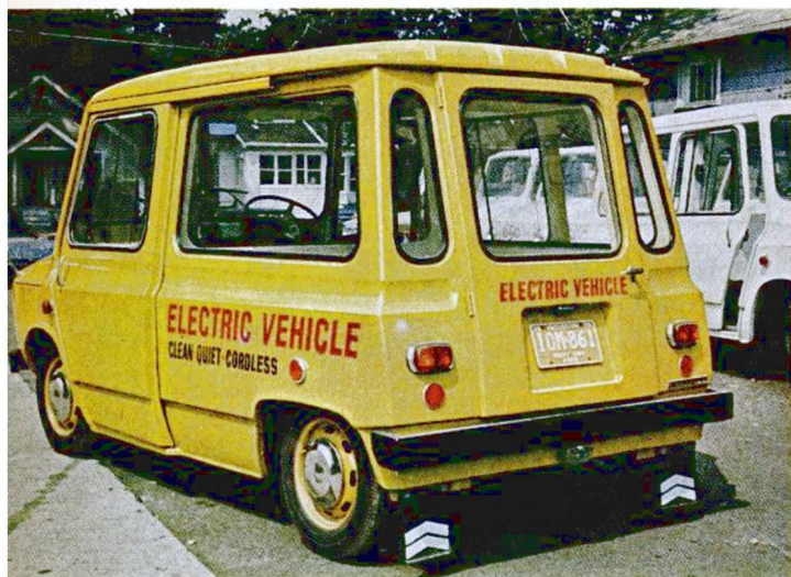
The EFP Battery Van runs on the power of 20 batteries. It has no clutch or transmission, and is reversed by a single toggle switch. Accelerator pedal selects from four battery combinations, and speed is maintained by constantly changing your foot position.
