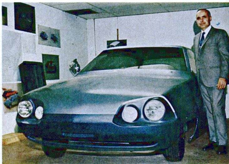
Full-scale mockup of the Voltair is shown by EFP president, Bob Aronson. The prototype of a 3,500-pound car with fiberglass body is now under construction. Its recommended top speed will be 90 mph, with a minimum range as high as 350 miles.
