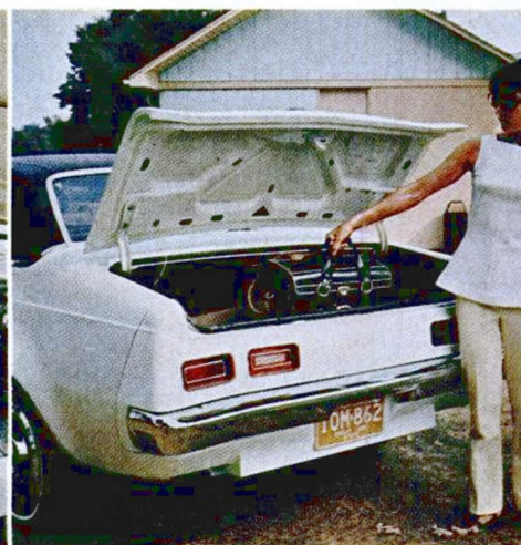
No trunk space was lost to batteries in the Hornet-bodied EFP Electric. They're stored up front, under the rear seat, and in a well below trunk. Curb weight is 5,300 pounds.
