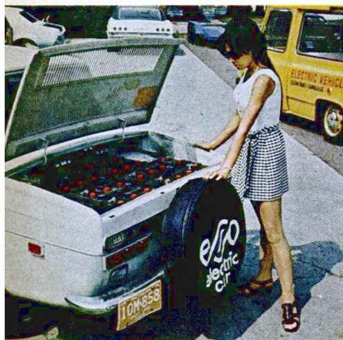
Batteries in the Mars II are stored where Renault 10's engine used to be—and also in front trunk. Mars II batteries weigh 1,900 pounds, raising vehicle's weight to 4,160.
