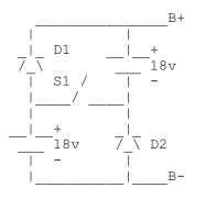
With S1 open, the batteries are in parallel -- you get 17v between B+ and B-. Each has a diode in series, so you lose about 1v (silicon) or 0.5v (Schottky). You can load the parallel batteries (draw current from them to run a motor), but can't do regen or charge them in parallel (because the diodes block reverse current flow).
