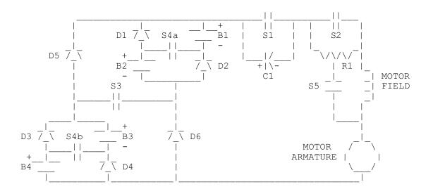
B1-B4 are your four 12v batteries. S1 is your main contactor, and has capacitor C1 across it as a snubber. R1 is your starting resistor, and S2 is the bypass contactor for it.
