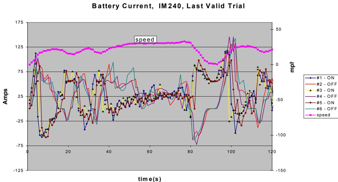
Figure 5. First half of cycle, dramatic differences are seen between the battery currents of the non-capacitor car and the capacitor version.
