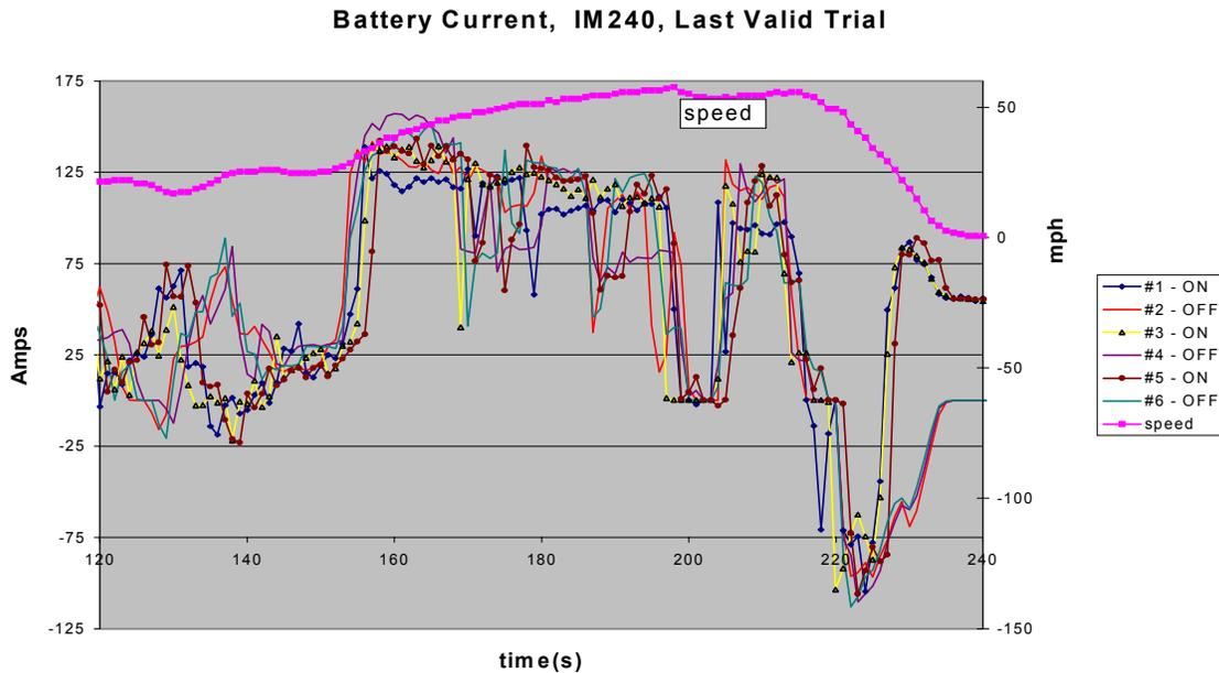
Figure 6. Last half of cycle, capacitor is depleted of energy; little difference thereafter
