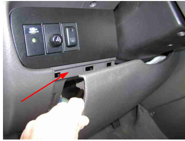
Pull top left to release panel and then remove set aside.
