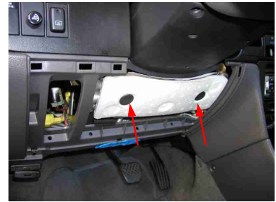
Pry out plastic pins. This is a slowest part of the task.
