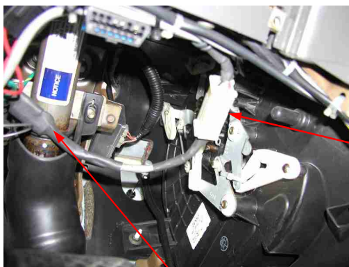
AH Filter and resistor as observed in my vehicle
